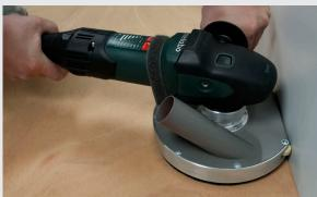
The freely rotatable suction hood enables the best possible suction and great freedom of movement when sanding edges.
